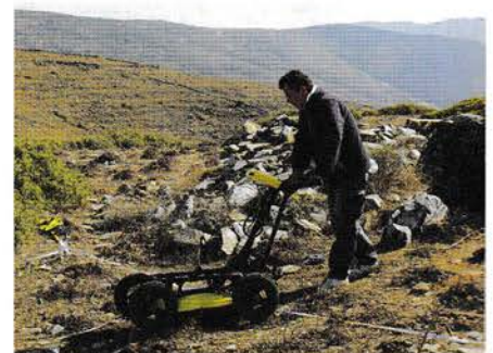
Apostolos Sarris pushing the Ground Penetrating Radar cart Zagora (photo: Irma Havlicek).
